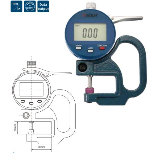
• Thickness gauges are attachment to the dial indicators and offer a quick and efficient means with a convenient grip handle to measure the thickness of paper, leather, rubber, fabric, metal plate, glass, plastic plat, etc
