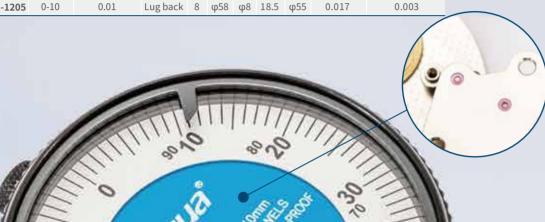
Jeweled bearing can reduce the friction, making higher sensitivity and quick response
